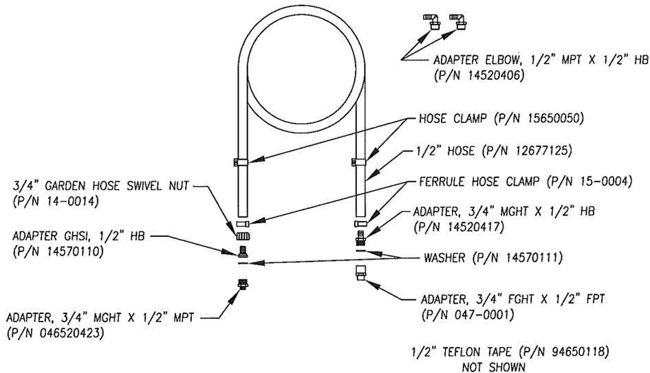
NOTE: CUSTOMER TO CUT HOSE AND INSTALL HOSE CLAMPS AS REQUIRED.
