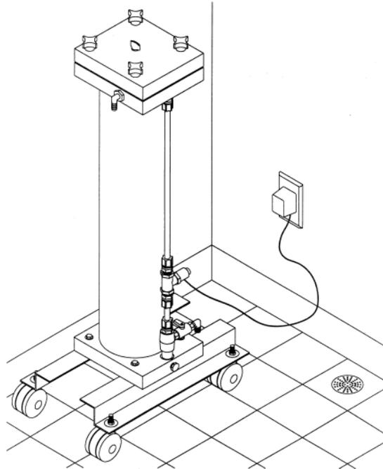
3. It is recommended to install cut-off valves on the inlet and outlet sides of each unit to facilitate changing of resin packs.
