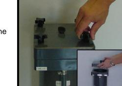
**3.** Remove the cover plates by unscrewing the black knobs located at each corner of the cover plates.
