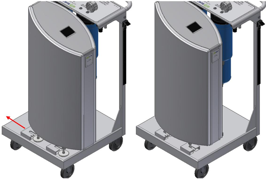
3. Place the locking pin in the hole on the cart to secure the left front foot of the Centurion to the cart.
