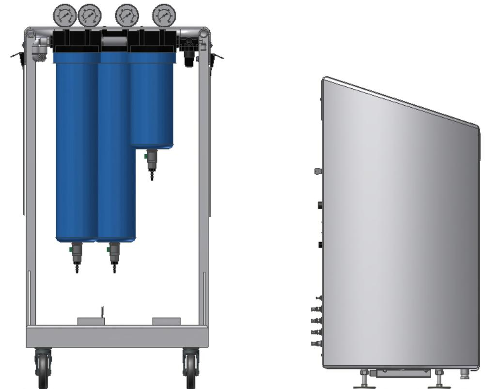
2. Carefully lift the unit (may require 2 people) onto the cart. Slide the feet into the feet mounting brackets on the Centurion.
