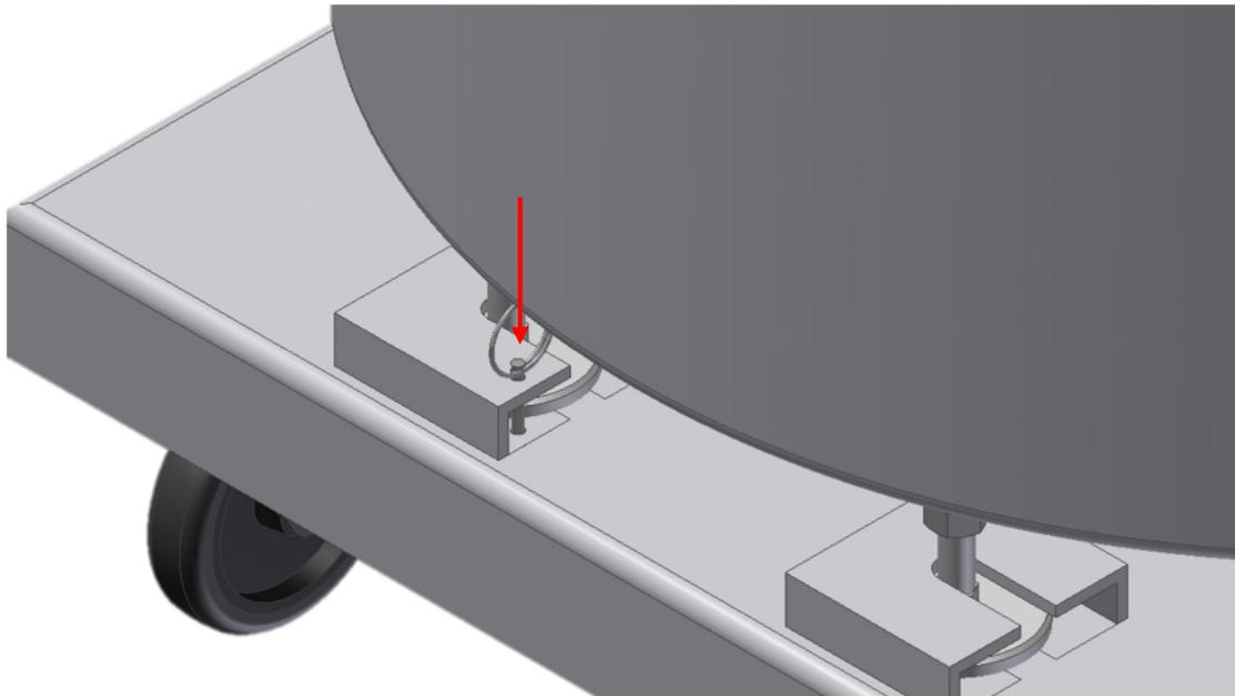
4. The Centurion should be mounted to the cart as shown in the following figures.
