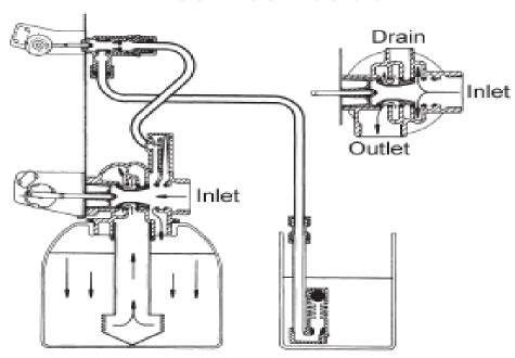
Hard water enters unit at valve inlet and flows down through the mineral in the mineral tank. Conditioned water enters center tube through the bottom distributor, then flows up through the center tube, around the piston, and out the outlet of the valve.
