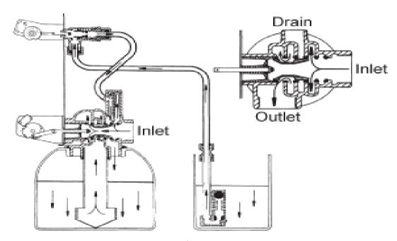
Hard water enters unit at valve inlet, flows up into injector housing and down through nozzle and throat to draw brine from the brine tank, brine flows down through mineral and enters the center tube through bottom distributor and out through the drain line.
