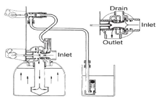
Hard water enters unit at valve inlet, flows through piston, down center tube, through bottom distributor, and up through the mineral, around the piston and out the drain line.
