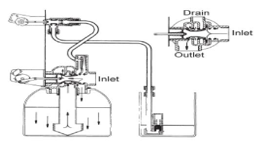
Hard water enters unit at valve inlet, flows directly from inlet down through mineral into center tube bottom distributor and up through center tube, around piston and out through the drain line.
