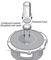
Do not scratch or chip polished ceramic face. Also . . .do not touch polished surface
