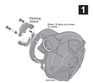
• Unfasten hardware holding Packing Gland in place and slide back on shaft to expose packing rings. A split Packing Gland is shown.
