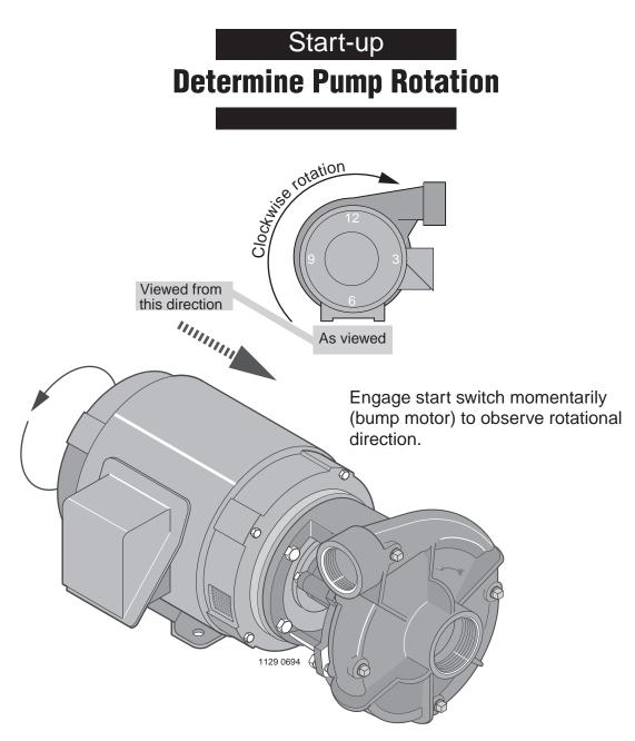
Direction of Pump Rotation is determined by viewing liquid end of pump from the **back** or **shaft side**, and **not** from looking into the impeller eye or front of volute case. A rotation direction arrow is cast into the pump body and shows correct rotation.
