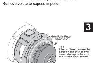
Install a standard gear puller to shaft end and impeller, placing puller fingers behind impeller vanes as shown.
