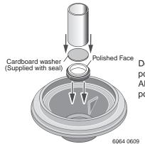
Do not scratch or chip polished ceramic face. Also . . .do not touch polished surface
