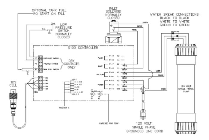
Figure 1.2 SRO Controller Diagram
