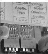
Example: If motor nameplate service factor amps = 3.3 A for 1AB2 or 5.3A for 2AB2, set motor overload switches as indicated.
