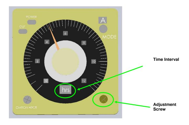
Once all validation of your set-up is complete, you must re-set the timer to 5 hours to meet the AAMI standards.
