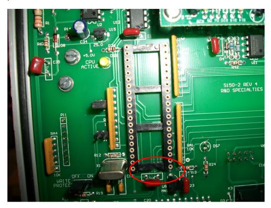
The empty socket is shown above. Note the orientation of the notch at the bottom of the socket. The replacement chip will have a notch to ensure that the CPU is keyed properly to allow proper operation. FAILURE TO ORIENT THESE IN THE SAME DIRECTION WILL LEAD TO DAMAGE TO THE CONTROLLER.
