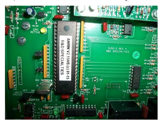
Verify that the pins on the replacement chip are aligned with the openings in the socket and gently press this into place. Ensure that the chip is fully seated in the socket.
