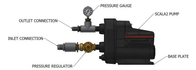
The pressure regulator is designed to reduce incoming water pressure. This regulator has a built-in thermal expansion bypass feature. This feature prevents downstream pressure from rising to more than 10 psi above the supply pressure.
