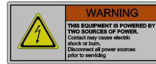
Equipment is powered by 2 sources of power. Risk of electrical shock
