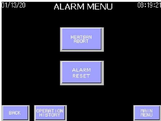
Within this screen, there are the options of aborting a heat disinfection cycle, resetting an active alarm, and viewing operation history. By pressing "**HEATSAN ABORT**" the unit will immediately go into a Cool down phase and return the system to STANDBY mode upon completion. The "**ALARM RESET**" will acknowledge an active alarm, clear it from the main screen and add it to the operation history.
