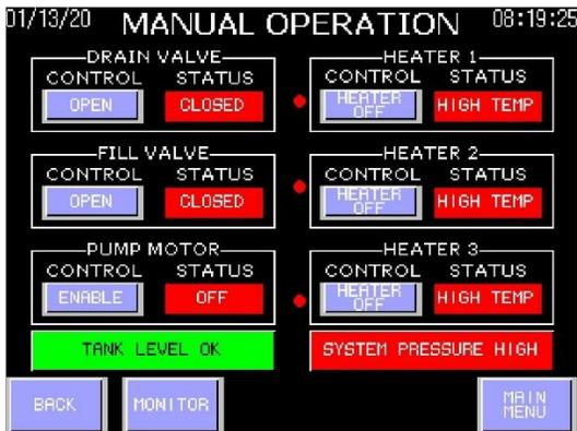
The **MANUAL OPERATION** screen gives you the ability to manually operate certain control components, when operated protection is still provided by any associated interlocks and safety control devices.
