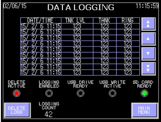
When you are ready to clear the data from the HMI, simply depress the "**DELETE LOGS**" button in the lower left corner of the screen.
