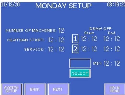
Firstly, enter the "**NUMBER OF MACHINES**". This indicates the number of dialysis machines that will take water for disinfection on this day. Next, enter the "**HEATSAN START**" time. To change the time, select each digit to be changed individually. A pop-up number keypad will appear on the screen, select the correct number and press "**ENTER**".
