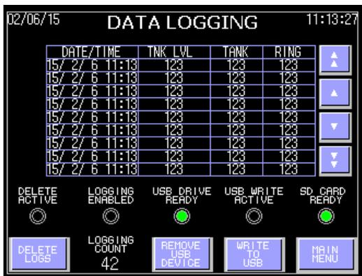
Install a USB drive into the port on the front of the control panel. The USB must be FAT 16 formatted. After a short period of time, the **USB DRIVE READY** light should illuminate green and the "**REMOVE USB DEVICE**" and "**WRITE TO USB**" buttons will appear.
