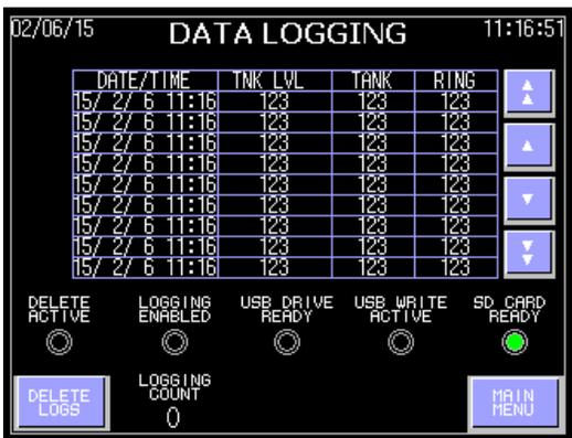
Once the information has been deleted, the logging count displayed on the bottom of the screen will be "0".
