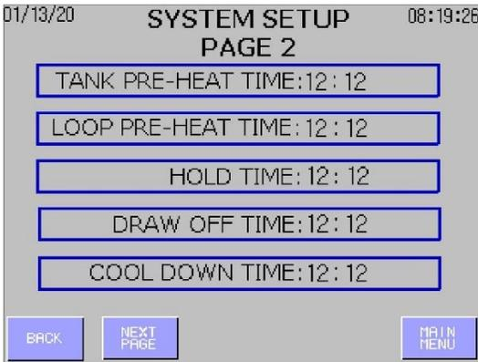
Enter the **HOLD TIME**. This time represents the time the distribution loop is held at the entered sanitization temperature. The minimum default hold time can be found in Section 6.9.
