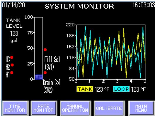
The "SYSTEM MONITOR" screen displays both tank level, tank and loop return temperatures. Press "MANUAL OPERATION" to go back to MANUAL OPERATION screen.
