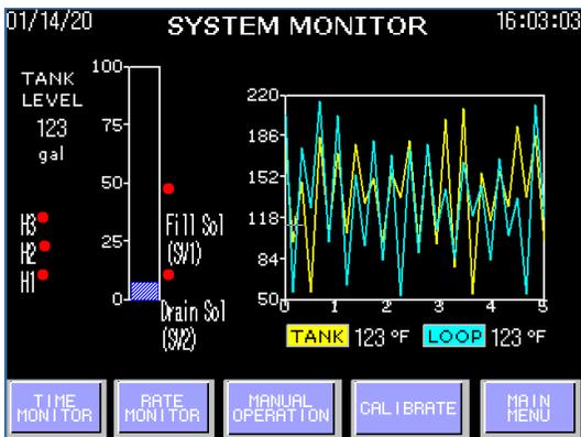
This screen will display information relating to the tank level in the form of a bar chart and actual volume reading in gallons.
