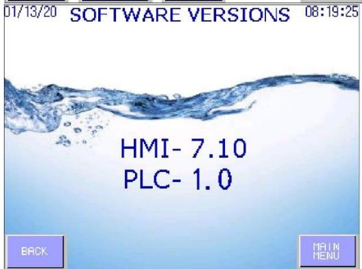
Details current software versions loaded on to the HMI and PLC. These will automatically update every time new code is uploaded into the unit. Press the **"BACK"** button to return to **FACTORY SETUP PAGE 6** screen or **"MAIN MENU"** to return to the **MAIN MENU**
