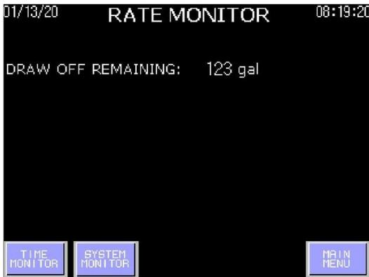
On selecting "**RATE MONITOR**" the **RATE MONITOR** screen will be displayed and will indicate the volume of water remaining for the disinfection of the dialysis machines. Press "**MAIN MENU**" to return to the **MAIN MENU** or press "**TIME MONITOR**" to gain access to time information or press "**SYSTEM MONITOR**" to return to the **SYSTEM MONITOR** screen.
