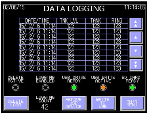
The **USB WRITE ACTIVE** light will illuminate orange while data is being written to the USB drive. Do not remove the USB drive while this is illuminated.
