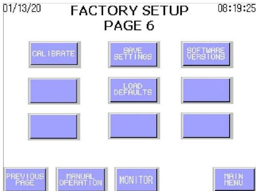
To save default settings press **"SAVE SETTINGS"** button for 5-10 seconds until you hear a single **"beep"**. This will overwrite previously saved settings.
