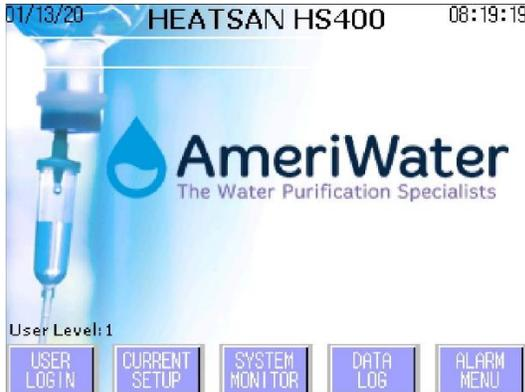
Log into the system at level 1 or higher. Upon returning to the **MAIN MENU**, you will have access to the "**DATA LOG**" button. Press this to go to the **DATA LOGGING** screen.
