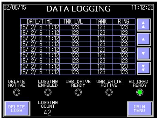
The **DATA LOGGING** screen will have a green light in the lower right corner that indicates **SD CARD READY**. If this is not illuminated, contact AmeriWater for assistance.
