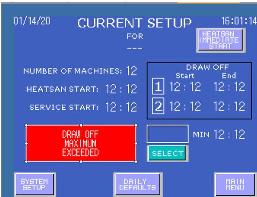
**NOTE:** If excess water is drawn off, a message of **DRAW OFF MAXIMUM EXCEEDED** message will be displayed as shown.
