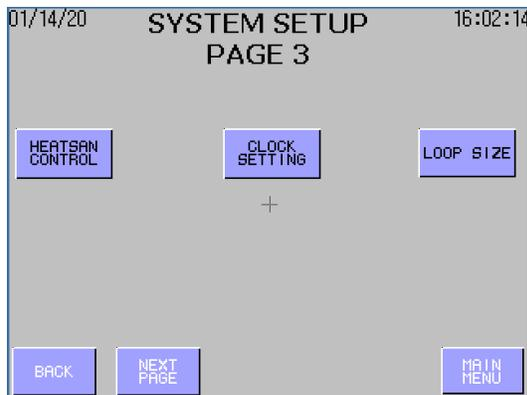
In this final set up screen you will be able to change the date and time settings, by pressing "**CLOCK SETTINGS**". This will take you to **TIME SETTING AND DISPLAY** screen. The clock is a 24hr clock. The date is displayed as mm/dd/yyyy. Press X in the upper right corner of the window when finished.
