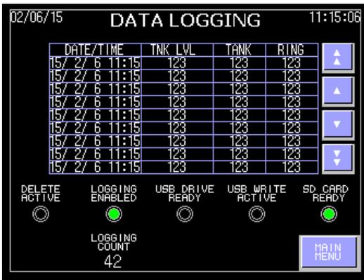
While the Heatsan is in **OPERATION**, the **LOGGING ENABLED** light will be illuminated green. While this is on, the "**WRITE TO USB**" or "**DELETE LOGS**" button will not be available.
