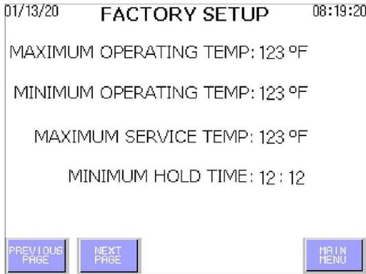
The unit will already have been programmed with a set of factory default values. Details of these can be found in Section 6.9. To change any values simply press the relevant digit, a number keypad will be displayed, select the desired value and press **"ENTER"**.
