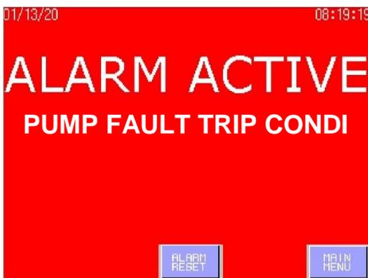
A secondary message will appear and scroll giving more details of the alarm condition. Users with Level 1 or 2 access can reset / acknowledge the alarm. Only users with Level 3 access can clear the alarm record from the event log by depressing the "**ALARM RESET**" button.
