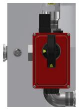
Figure 22 Concentrate to Drain Valve
